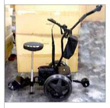
This remote control golf trolley has a 28AH battery able to cover the distance to play 18 holes. Easily folds away, has easily removable wheels, and a cover for the electric motor and controller unit. This will help prevent corrosion and damage due to impact with other objects.
